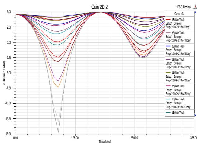
Fig 10: 2D gain plot for 2.08 GHz frequency
