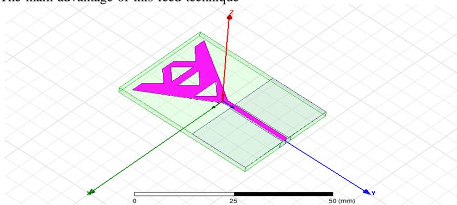
Fig 6: Geometry of the patch antenna
